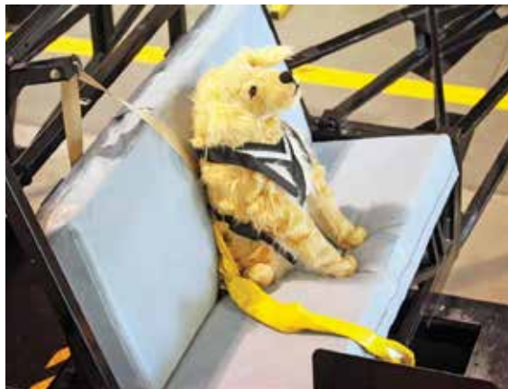
The CPS developed three crash-test-dummy dogs; the largest is this 75-pound “Golden Retriever.”
