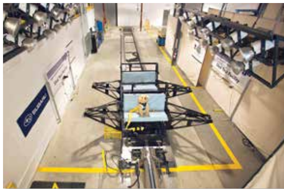
A crash-test-dummy dog (and a multitude of cameras) all set for a Center for Pet Safety (CPS) restraint test.
