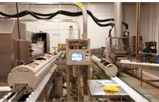
One of the HPP facilities operated by American Pasteurization Company, of Milwaukee, Wisconsin. Those round, cradle-like tubes on the left are fully loaded with sealed packages of food, and are ready to enter the HPP tank on the left side; the tubes on the right side are empty and awaiting product.
