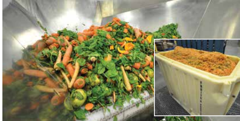
Fresh fruits and vegetables enter a grinder at Champion’s produce supplier; this, too, is delivered to Champion in a slurry (inset).
