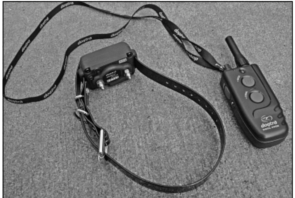
“Remote training collars,” controlled by radio signals, deliver electric shocks to a dog.
