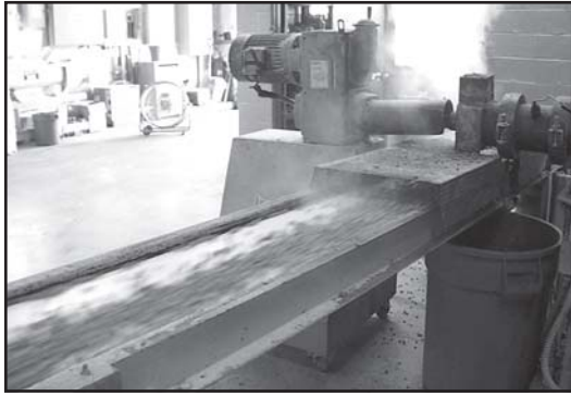
The manufacturing process is helpfully transparent in this tiny plant. Steam rises from the extruder and the freshly extruded food whizzing by on the conveyor belt, on its way to a dryer.
