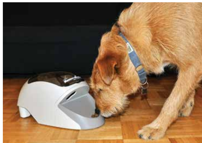
The Manners Minder (also sold under the name Treat & Train) was among the first remote-controlled treat-dispensing devices on the market. It enables a handler to deliver treats to a dog at a location that is up to 100 feet away – perfect for certain training applications. However, some dogs are afraid of the devices.
