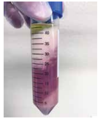
Centrifuging separates the tissues into layers; the top two (oily and white) are discarded. The red fluid and grey mass at the bottom are removed to a new tube.
